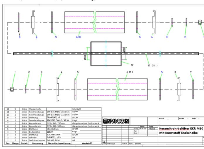
Version with stainless steel end discs (exploded drawing)
